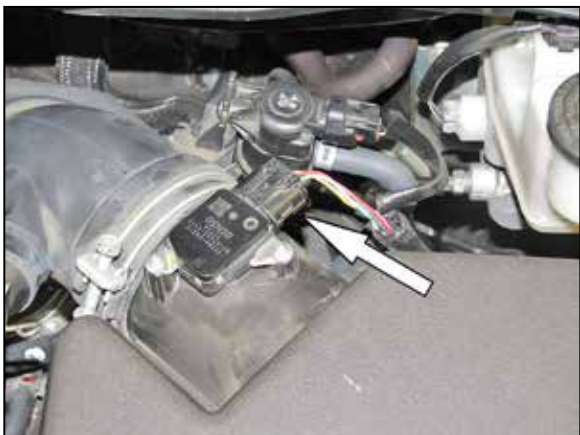
2. Disconnect the mass air sensor electrical connection.
