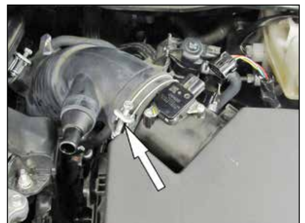
5. Loosen the hose clamp securing the intake hose to the air box lid.
