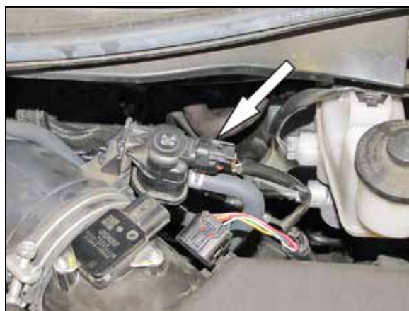
3. Disconnect the EVAP solenoid electrical connection.
